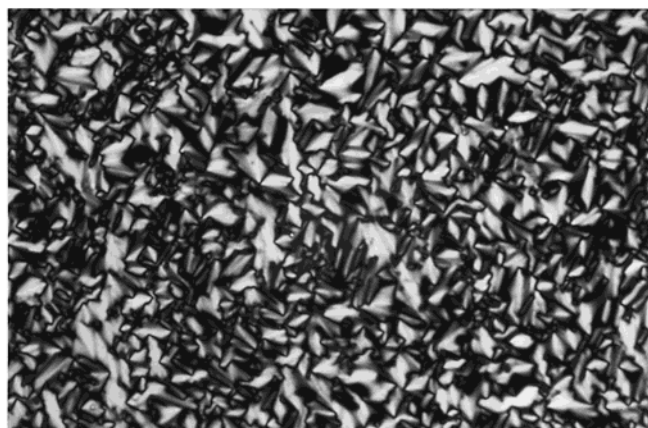
Figure 3. Optical micrograph of the fan-shaped texture of poly(3) at 93 °C (original magnification 320×).
